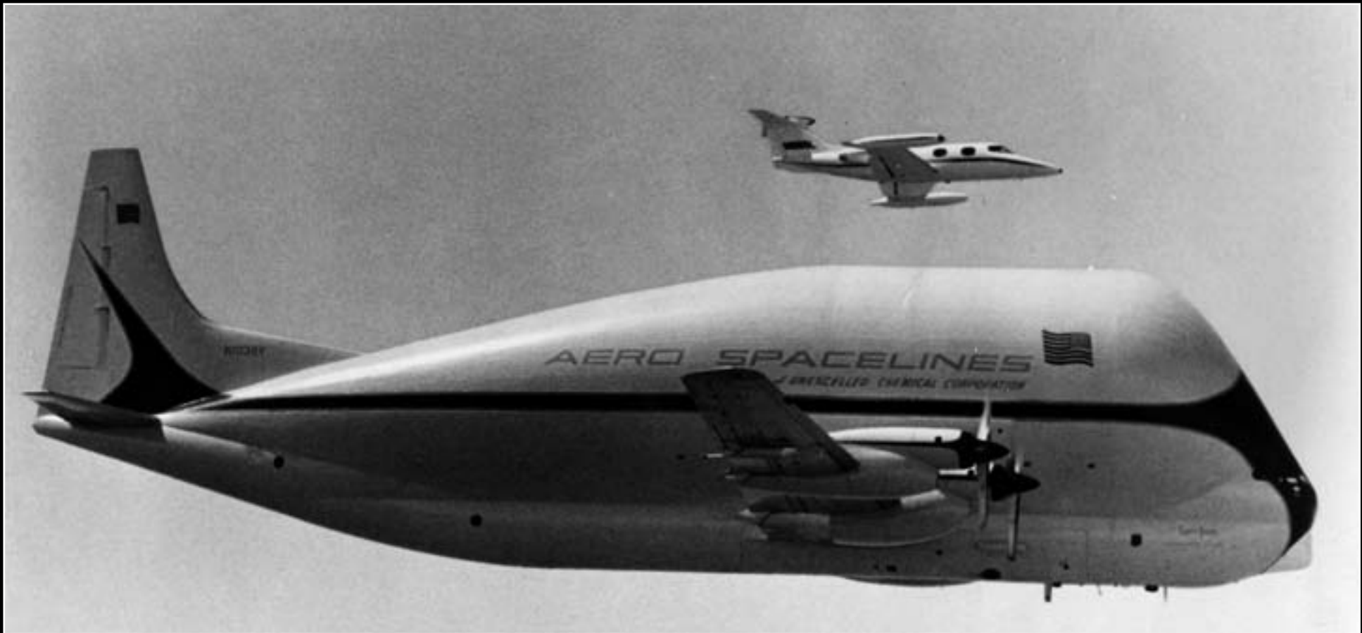
Clay pilots a Lear 23 above Aero Spacelines, Inc.'s Super Guppy, the successor to the Pregnant Guppy, used to ferry oversized cargo components circa 1962.
